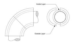
**SMC's High Temperature Molded Double Layer Perlite Fitting Covers** use two individual fitting covers nested over one another. The inside layer, the fitting cover in contact with the pipe, will be a 3" thick fitting. The outside layer will range from 2 ½" to 5" in thickness, depending on total thickness required. Whenever possible, SMC staggers the insulation seams to deter direct heat loss and water penetration into the insulation system.
